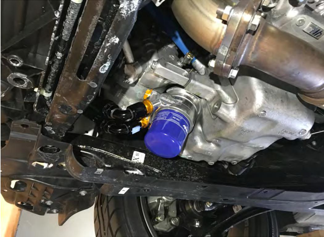
2.3 Measure and mark the factory bumper reinforcement beam for the mounting holes for the oil cooler core as shown. (57mm from side and 26mm from front)
