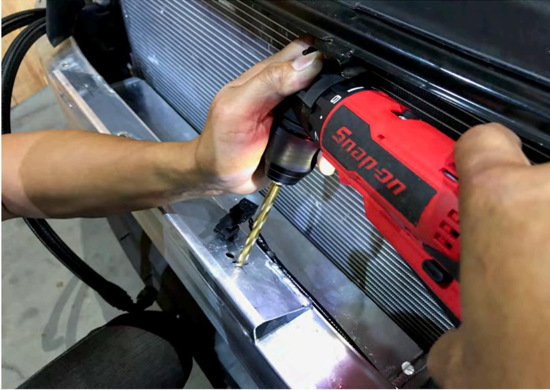
2.5 Cut a 2" hole on the factory plastic air duct panel on the passenger side next to the condenser as shown.
