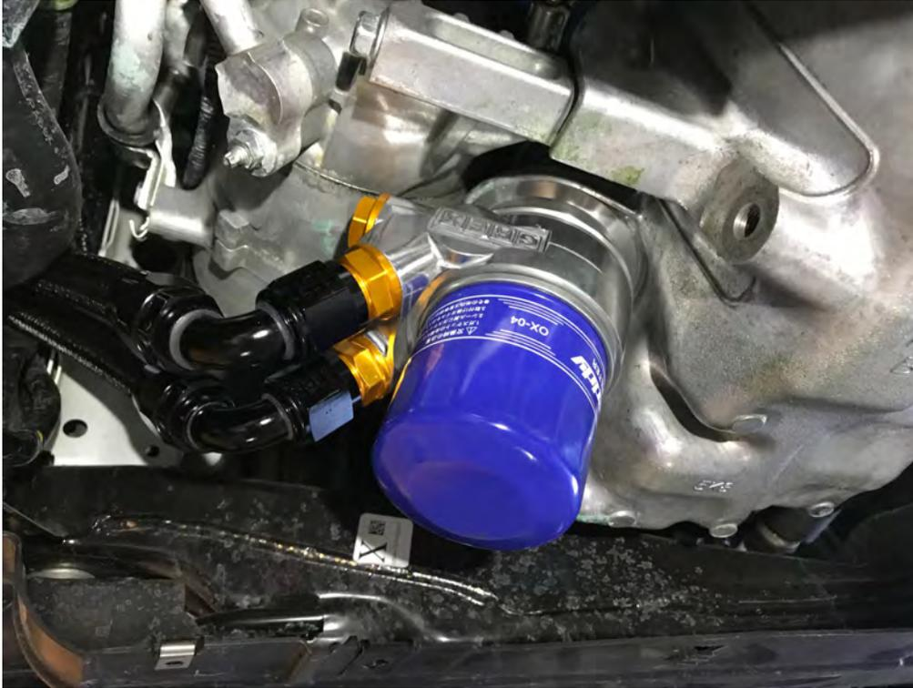
2.8 Lube the o-rings on the ORB fitting and secure the Oil Line #1 and #2 to the core side. 90deg ORB to the driver side and 120deg ORB to the passenger side.
